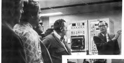
"by tape command, the machine can change 16 tools"
